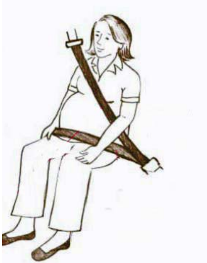
Figure 10 NHTSA Recommended Lap Belt Position
